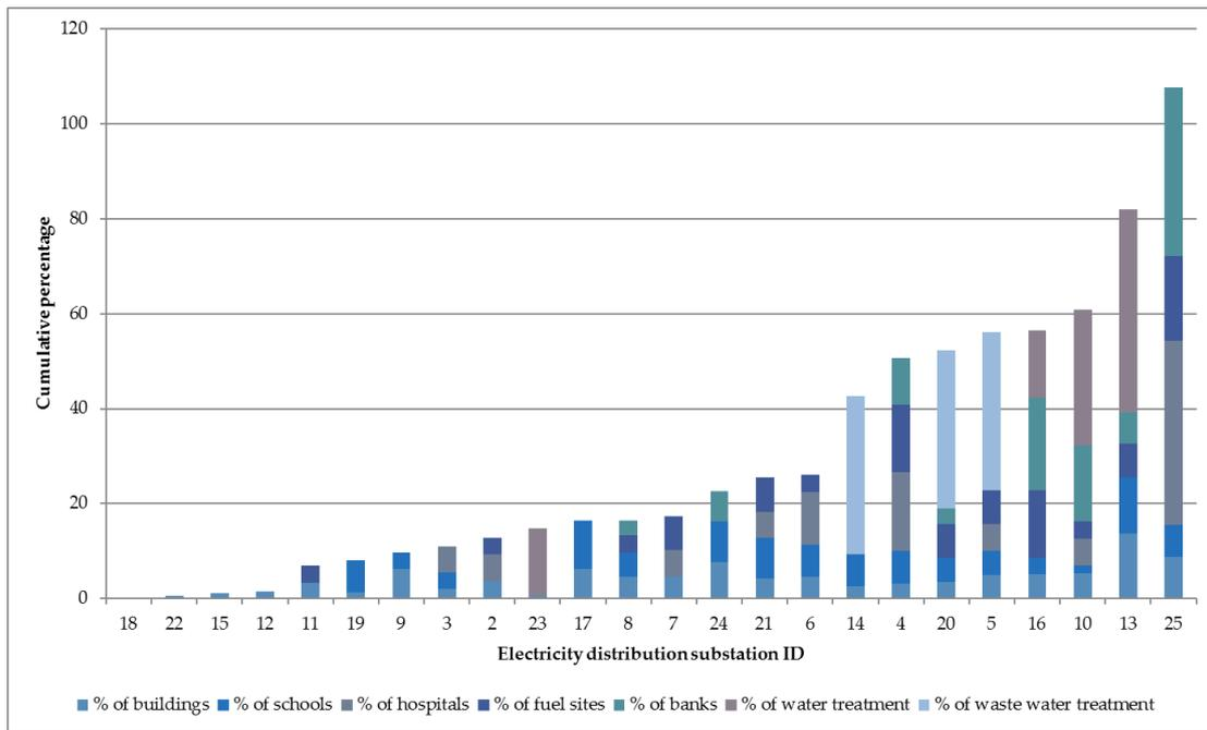
**Figure 44: Vulnerability plot showing the magnitude of direct and indirect failure consequences for electricity distribution substation assets (sink assets)**
