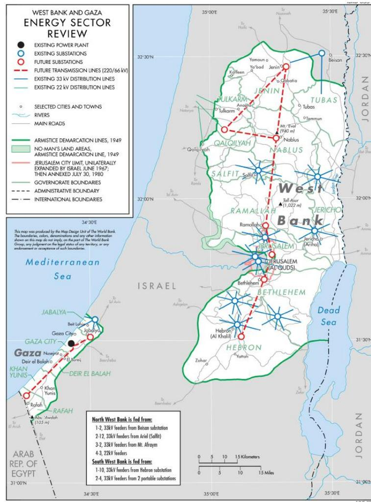
Figure 66: Current and proposed electricity supply system in the West Bank and Gaza (UNISPAL 2007)
