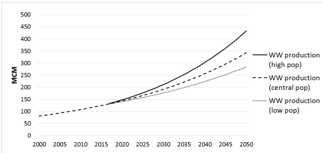
Figure 80: Projected wastewater production (MCM) based on current levels of production per capita (PWA 2012)
