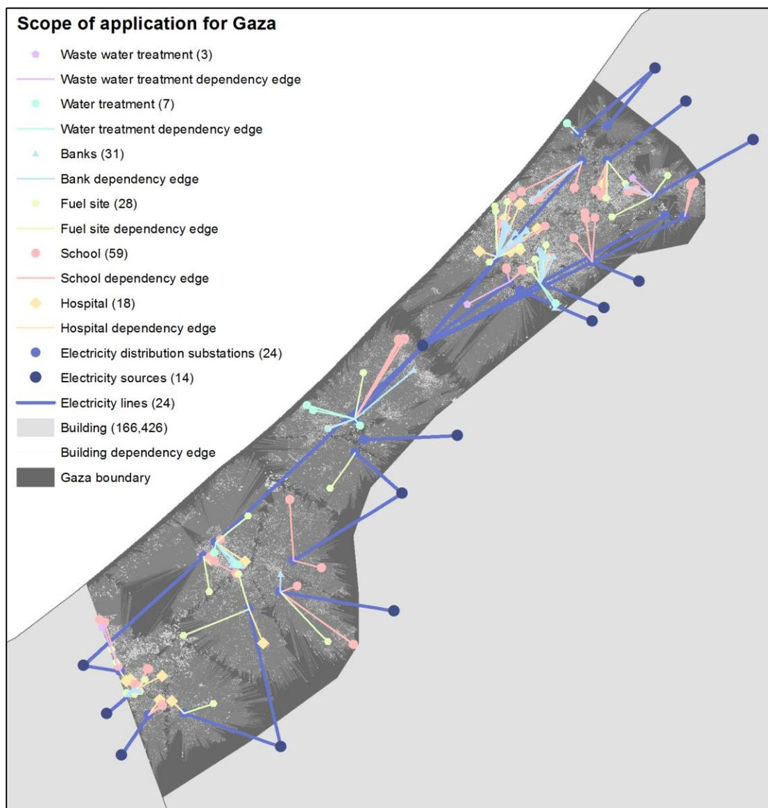
**Figure 43: Scope of the application for Gaza, showing the electricity network and a range of dependent assets from the energy, water treatment, waste water treatment, health, banking and education sectors. The number of assets of each type is indicated in the figure legend**
