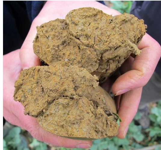
Figure 4 - Characteristic mottling in seasonally-waterlogged gley soils. (Northamptonshire. S. Hallett )
