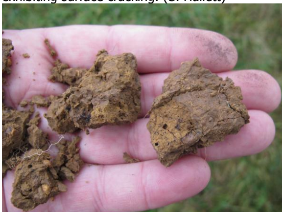
Figure 3 - Slickensides, or clay shear plates. ( S. Hallett )
