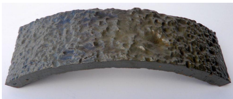
Figure 8 - Characteristic pitting in water mains pipe due to soil-water corrosion. ( S. Hallett )
